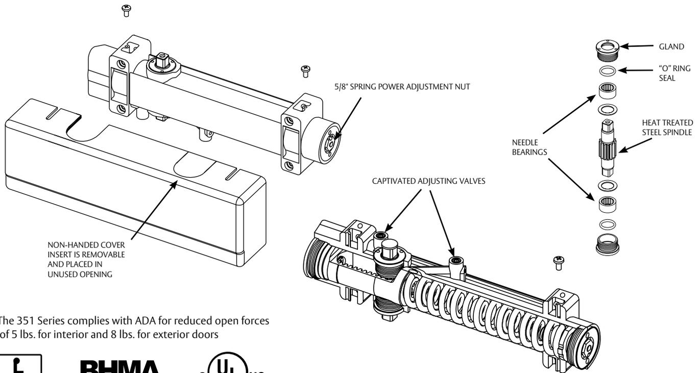
The 351 Series complies with ADA for reduced open forces of 5 lbs. for interior and 8 lbs. for exterior doors
