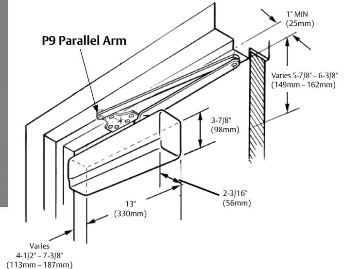
Parallel Arm Applications - The 351 closer is mounted on the push side of the door. As the door opens, the closer swings with the door and gives full headroom in the door opening. Other advantages: the closer arm does not project into the room; the frame can be quite narrow and the door can be swung open much farther than in Top Jamb Applications.
